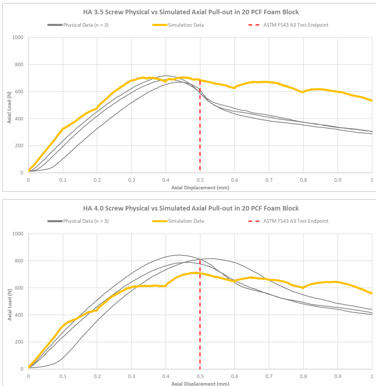
Figure 5. Load-displacement curves from the physical experiment (n = 3) and the simulated (half-sized grid) axial pull-out tests of HA 3.5 (top) and HA 4.0 screws (bottom) in 20 PCF polyurethane foam blocks up to 1 mm pull-out displacement
